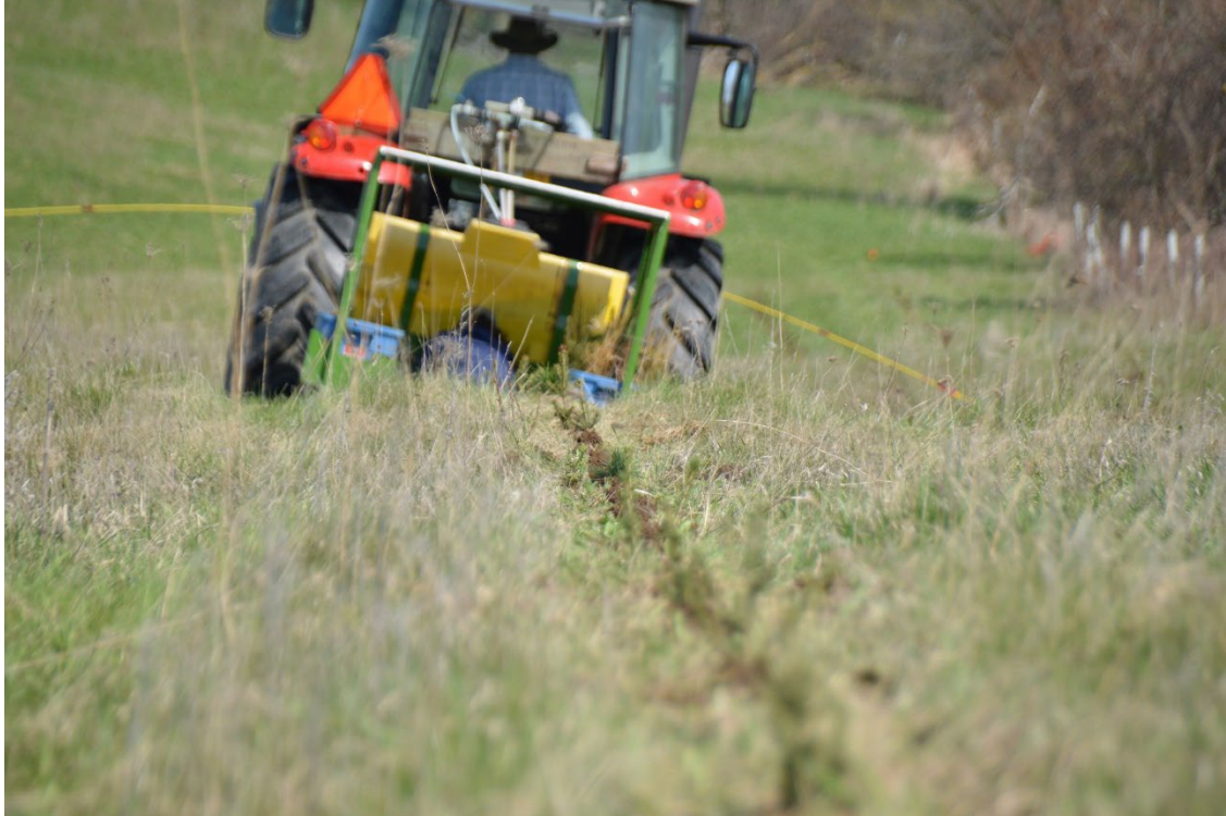
A row of seedlings planted by a tree planting machine. Tree planting machines are used in flat and dry areas.
